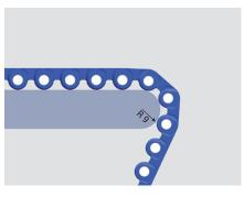
**Turning** in scarcely **18 mm**, the frozen products that stick to the belt will detach without the need to use scrapers.
