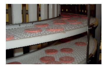
EUROBELT plastic modular belts can be easily moved, removed, lifted, and even disassembled, in order to reach those parts that are hard to access or clean.
