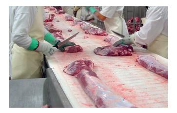
As belts are manufactured using plastics with a minimum absorption rate, they do not absorb smells or retain bacteriological contamination, after being properly washed.
