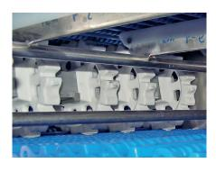
The exclusive opened sprocket of Series B50, with rounded edges and without any corner in its toothed crown, enables to have access to all its surface, achieving a complete cleaning.
